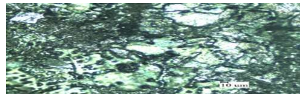
Fig.4 Mg-MMC with 2% B 4 C & 3% MWCNT by wt
