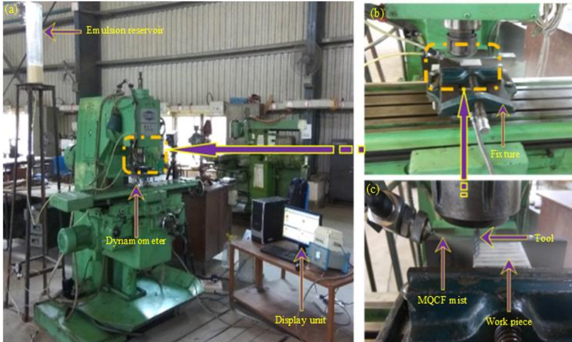
Fig. 1. (a) Overview of experimental setup, (b) workpiece
