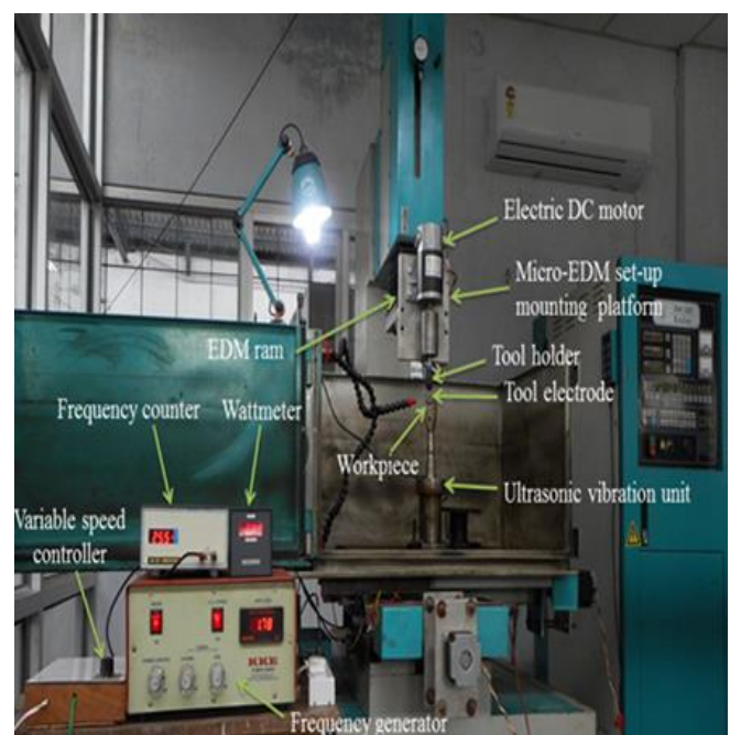
Fig. 1. Photographic view of developed Drilling ultrasonic assisted Micro-EDM setup
