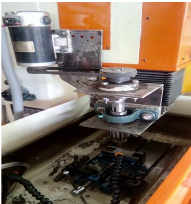
Figure 2. - EDFG setup assembled on EDM machine
