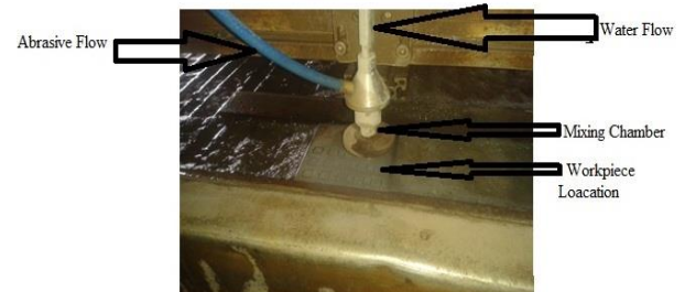
Fig. 1. Abrasive water jet machining during machining of Hastelloy C276
