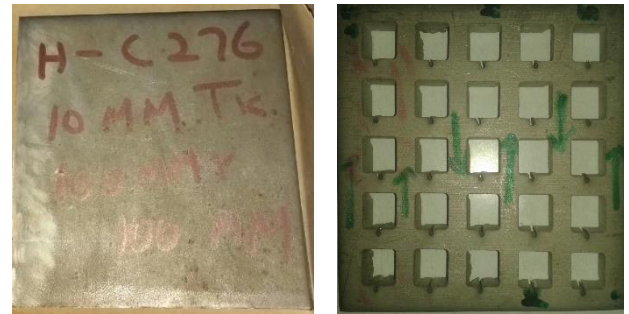
Fig. 4. Hastelloy work piece Before & After Machining.
