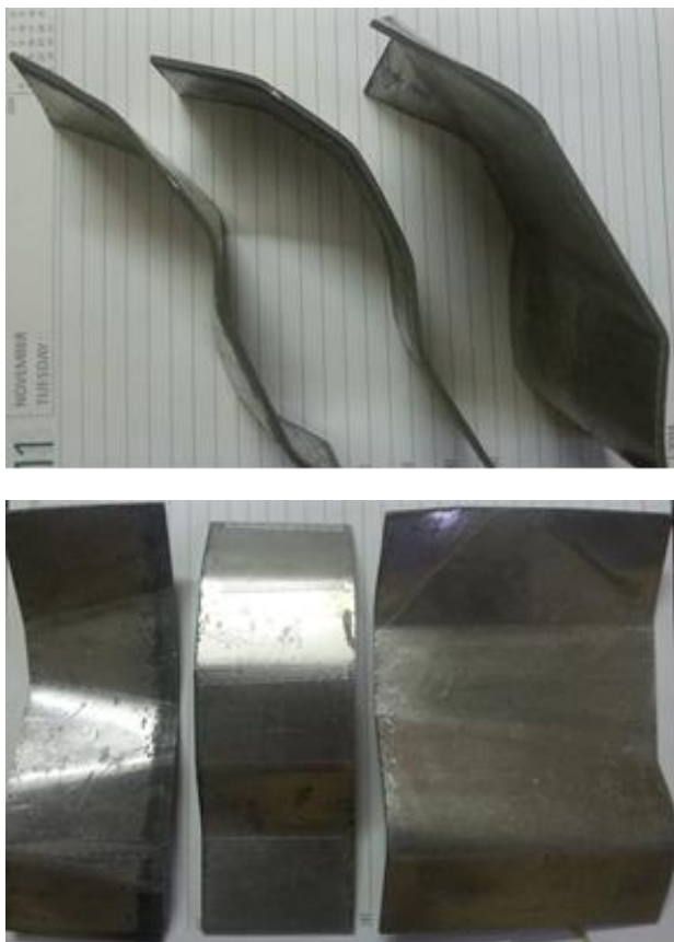
Fig. 11 Sheet metal components with complex geometries
