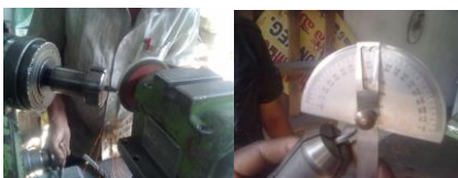
Fig.2 Alteration of drill geometry using tool & cutter grinder
