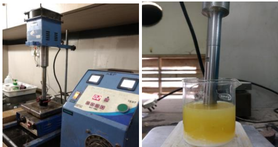
Fig.2 a) Ultrasonicator b) magnetic stirrer
