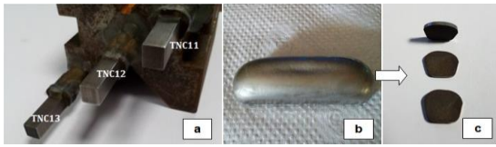
Fig. 1. (a) Rectangular profile for kerf study (b) TiNiCu ingot bar (c) Surface roughness sample
