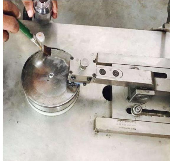
Fig.4 Pin on disc with a fixture for positioning chain pin
