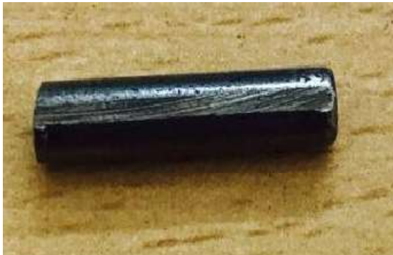
Fig.6 Wear pattern on the body of chain pin
