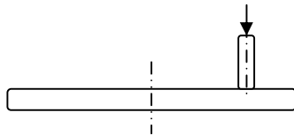
Fig.2. Schematic diagram of normal position of pin on disc
