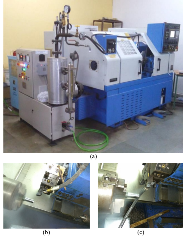
Fig. 1. (a) Steam generation device and supply of water vapour to machining zone through hose, (b) Water vapour supply through external nozzle, and (c) Water vapour supply through special tool holder
