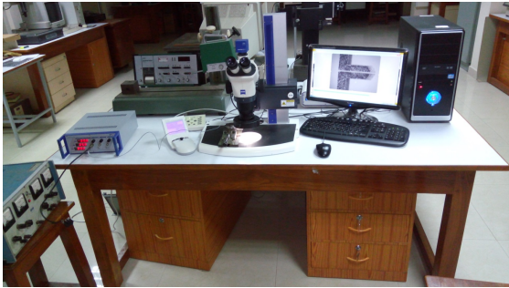
Fig.3 Experimental Setup that includes Power Supply, Amplifier, Piezo Actuator, Micro gripper and stereo microscope
