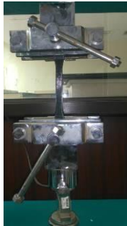
Fig. 9. ASTM D638 specimen for Tensile Test
