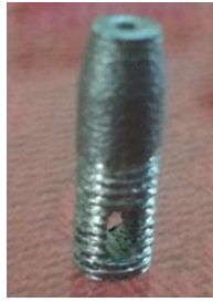
Fig. 8. Implant specimen fabricated by DMLS process
