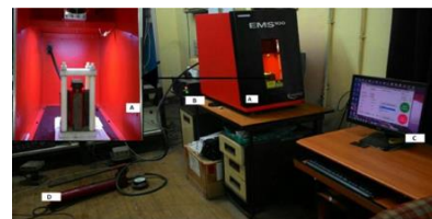
Fig. 1. Pictorial view of experimental set up: A. Work station; B. Laser beam delivery unit; C. Computer interface and D. Hydraulic pump with pressure gauge
