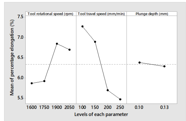
Figure 6 Main effect plot for means of percentage elongation in 1 mm sheets
