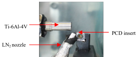
Fig. 6 Closer view of in-situ cryogenic micro turning setup
