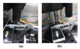
Fig. 9: (a) Initial position of confocal while measuring bending radius (b) Final position of confocal while measuring bending radius
