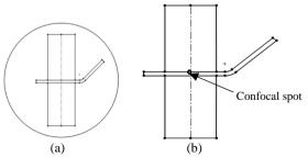
Fig. 4: Schematic diagram of (a) Plate arrangement shown at rotary table (b) Confocal spot shown at center of fixture
