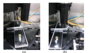
Fig. 1: (a) Plate arrangement shown before bending (b) Plate arrangement shown after bending
