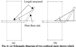
Fig. 6: (a) Schematic diagram of two confocal spots shown which are taken for measurement (b) Schematic of triangle formed.
