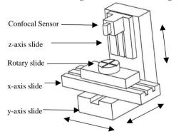
Fig. 2: Schematic diagram of Confocal mounted on z-axis slide with all 4-axis shown.
