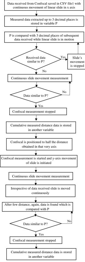
2. Through the movement of linear slide in x-axis up to half of the distance between A and B, confocal point is focused at midpoint. Now confocal point is moved vertically using y-axis slide until it touches the curvature which when measured is marked H.
