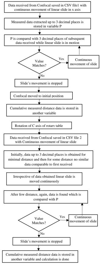
Fig 7: Flowchart of C# program for automated measurement of bending angle
