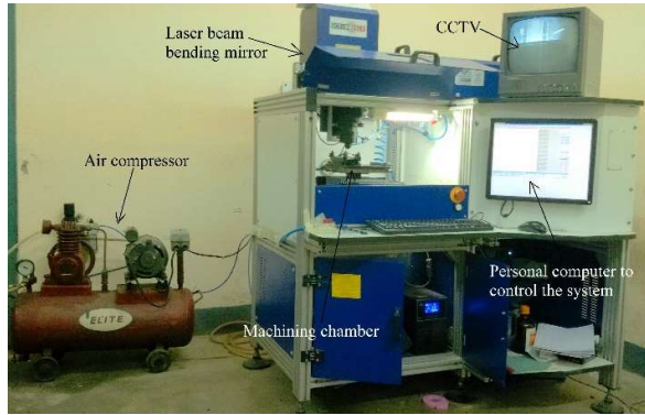
Fig. 1 Photographic view of the multi diode pumped pulsed fiber laser system
