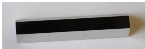
Fig. 10. DLC Coated Prismatic Guide way on Hardened Steel
