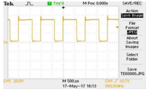
Fig. 3. 50V Rectangular pulsed voltage cycle with 1000Hz frequency
