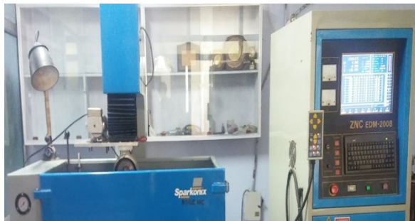
Fig. 2: Setup of Electrical discharge diamond grinding
