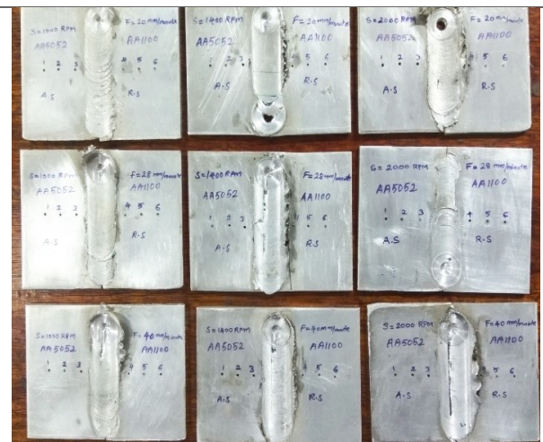
Fig. 3. Friction stir welded specimens
