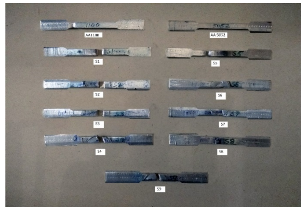
Fig.11. Failure location of tensile test specimens
