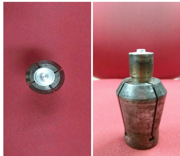
Fig. 1. FSW Tool and Collet
